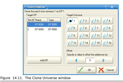
If cloning will overwrite patch information in the destination, you will be asked for confirmation. The console will only unpatch previous fixtures that are in the way of new ones; the rest of the destination universe will be untouched.
