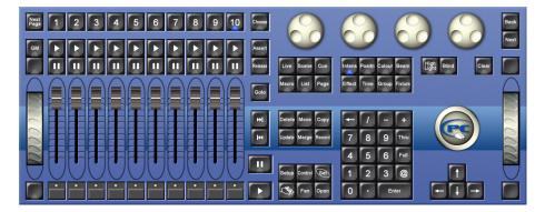
The front panel of Hog 3PC looks and behaves the same as a Wholehog 3 console. Click on buttons to simulate pressing keys on the console. You can also click and drag to alter the various encoders or faders. In addition, when you click and drag on the trackball, it will illuminate blue and your mouse will adjust the pan and tilt of the selected fixtures.
