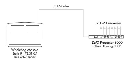
Example B: The console is a DHCP server, and all other nodes obtain an IP address from it.
