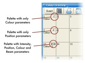
Figure 17.8. Example of Palettes containing different parameter types
