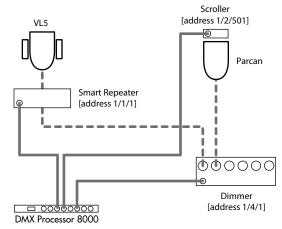
Figure 14.9. Examples of Fixtures requiring Multiple Patch Points
