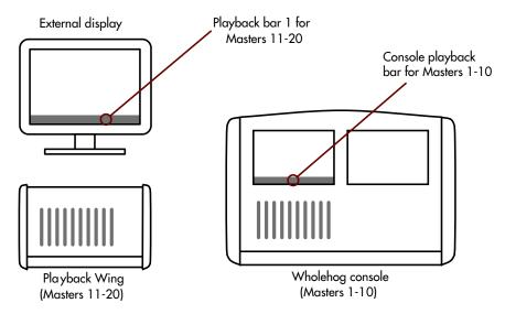
Figure 12.11. Docking Playback Bars with wings and external displays
