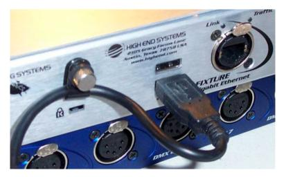
**V-Lock Style Locking Power Connector:** the DMX Processor 8000 ships with a special IEC cable with a locking power connector. In addition a standard IEC cable can be used.
